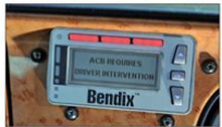
FIGURE 8 - IMPACT ALERT TEXT AND LIGHT PATTERN AS SEEN ON THE BENDIX® DIU
