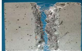
Keep in mind that if fiber is only used, the subgrade must be properly compacted and prepared in accordance with the geotechnical engineer's recommendations. Once any differential settlement occurs, the fiber will not prevent cracks from developing and increasing in width.
